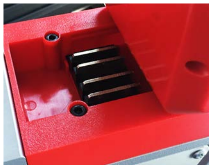
Beryllium contact points on the EBM.360
