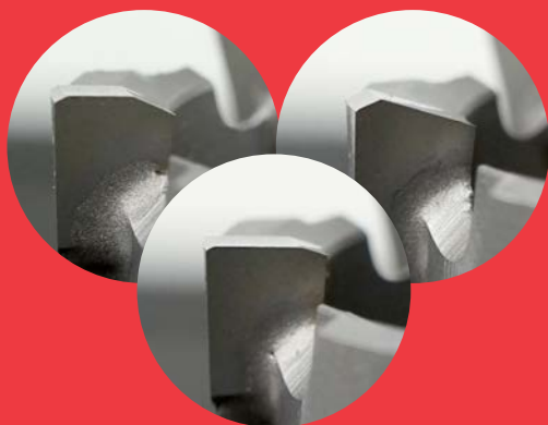
TCT has up to three different teeth
